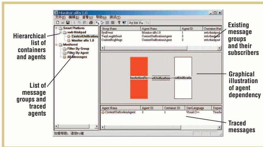
Figure 8. Monitor agent user interface. The system-level agent lets users remotely launch or kill an agent, trace agent messages, or send messages manually.
