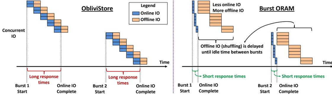
Figure 2: **Reducing response time.** Because Burst ORAM (right) does much less online IO than ObliviStore (left) and delays offline IO, it is able to respond to ORAM requests much faster. In this (overly simplified) illustration, the bandwidth capacity is enough to transfer 4 blocks concurrently. Both ORAM systems do the same amount of IO.
