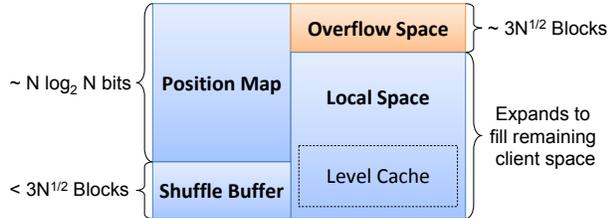
Figure 6: **Burst ORAM Client Space Allocation.** Fixed client space is reserved for the position map and shuffle buffer. A small amount of overflow space is needed for blocks assigned but not yet evicted (*data cache* in [24]). Remaining space is managed by *Local Space* and contains evictions, early shuffle reads, and the level cache.
