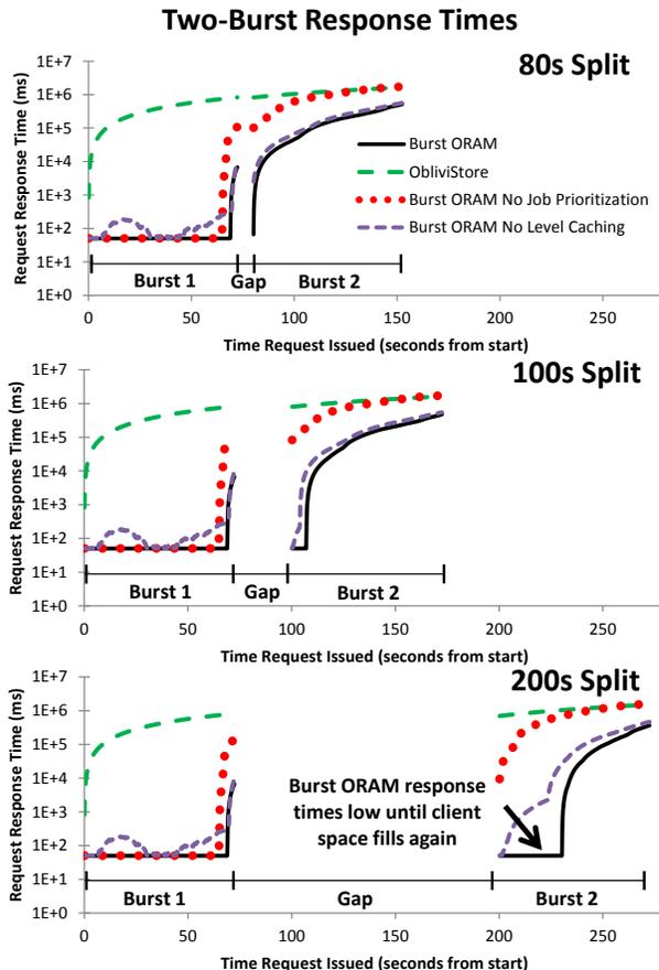
Figure 9: Response times during two same-size bursts of just over  $2^{17}$  requests spread evenly over 72 seconds. Client has space for at most  $2^{18}$  blocks. No level caching causes early spikes due to extra early shuffle reads.
