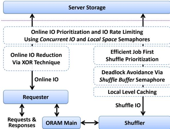
Figure 5: **Burst ORAM Architecture**. Solid boxes represent key system components, while dashed boxes represent functionality and the effects of the system on IO.
