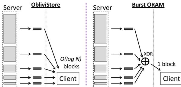
Figure 3: **Reducing online cost.** In ObliviStore (left) the online bandwidth cost is  $O(\log N)$  blocks of IO on average. In Burst ORAM (right), we reduce online IO to only one block, improving handling of bursty traffic.
